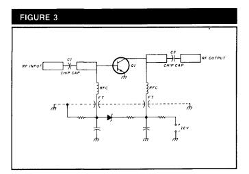
RF amplifier using 50-ohm microstrip.
