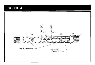
Layout of RF amplifier showing two strips of copper to be removed with an X-ACTO knife to produce a microstrip pc board. Cut away copper to mount DC blocking chip caps C1 and C2.
