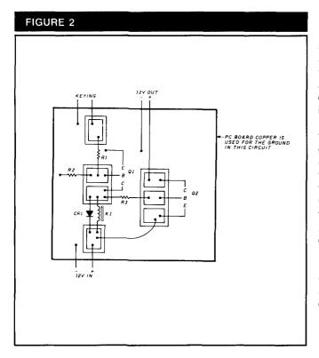
Board layout showing pads made by removing copper strips around each square using X-ACTO knife methods. A "score knife" could also be used to cut away the copper, leaving the isolated pads.
